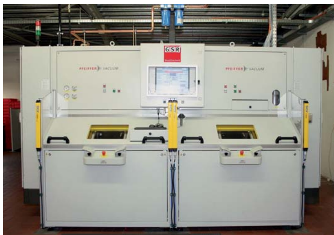
Fig. 4: Uniquely precise: The new leakage test stand for high pressure valves in the GSR test field
